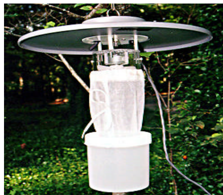
Photograph 2. New Standard Miniature Light Trap with CO 2 release (from J.W. Hock Company, 2005).
